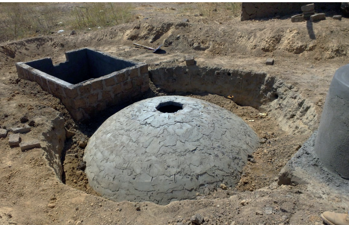
Figure 3. An improved model of an earth pit kiln in Southern Burkina Faso with improved control of airflow. Photograph by Markus Melin.
