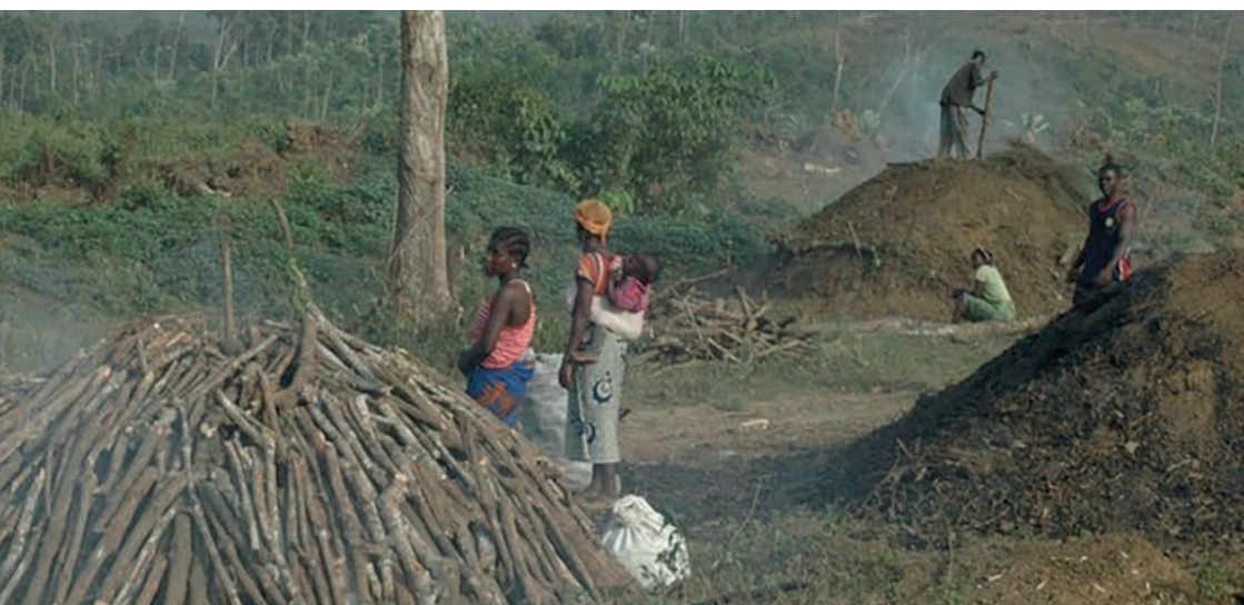
Figure 2. A traditional earth mound kiln shown with wood stacked (front left), covered (right) and lit (back). Photograph adopted from http://www.bbc.co.uk/news/world-middle-east-16598389
