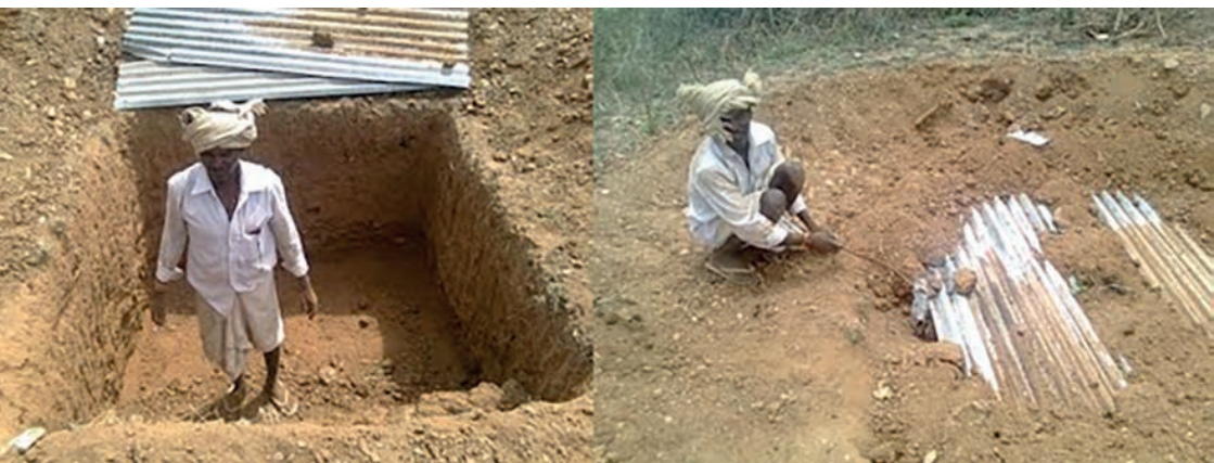
Figure 1. A traditional earth pit kiln open (left) and sealed with steel plate with wood inside (right). Small air-channels are made on top to allow outflow of emissions. Photographs adopted from http://biochar.bioenergylists.org/taxonomy/term/334
