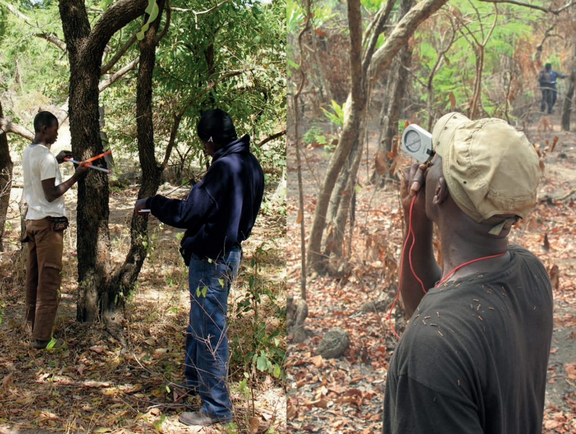
Figure 11. Field crew measuring and writing down tree diameters in Burkina Faso (left). A field crew member measuring tree height with a Suunto hypsometer in Sierra Leone (right). Photographs by Janne Heiskanen (left) and Markus Melin (right).
